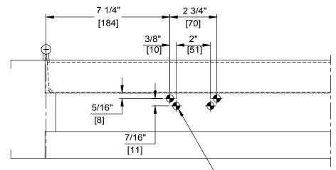
FOR 1/4-20 MACHINE SCREWS USE 7/32" DRILL FOR No.14 WOOD SCREWS USE 5/32" DRILL DPK FASTENERS DRILL 1/8" PILOT HOLE FOUR (4) HOLES IN FRAME FOR PA BRACKET
